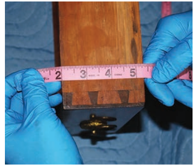
Three half-blind dovetails join the desk drawer sides to the front.
